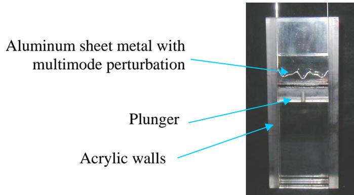
Figure 3. Test section for MR fluid/water interface.
