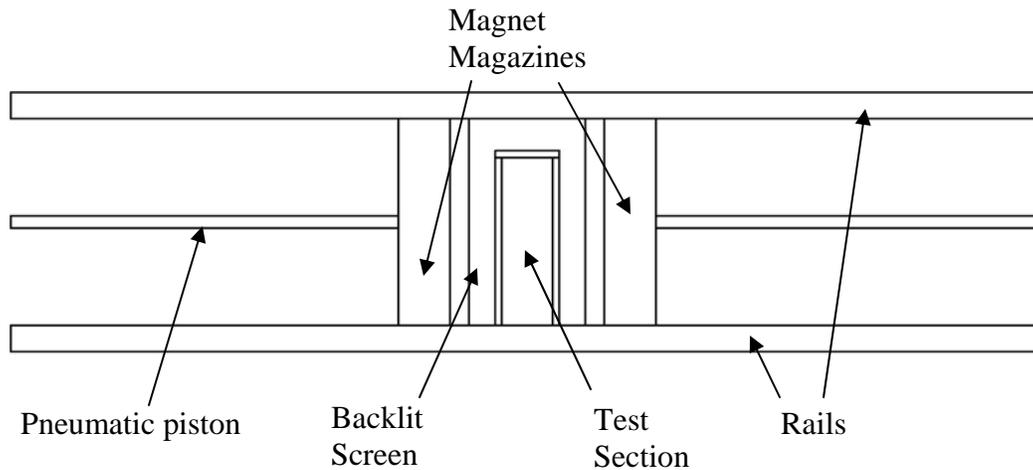
Figure 2. Side-view of the experimental setup.
