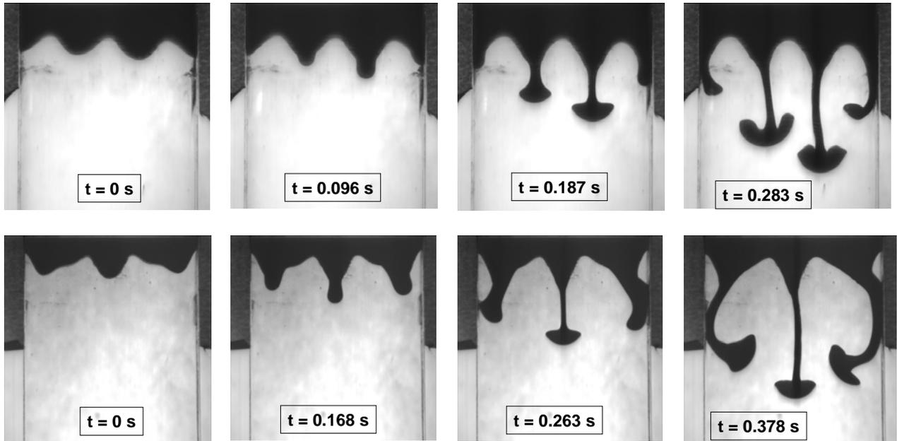
Figure 6. Top row is a montage from a single mode initial condition experiment and the bottom row is from a multimode initial condition.
