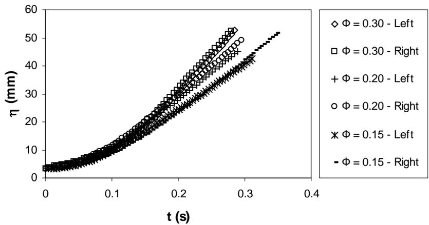
Figure 10. Measured growth rates for all three mixtures.
