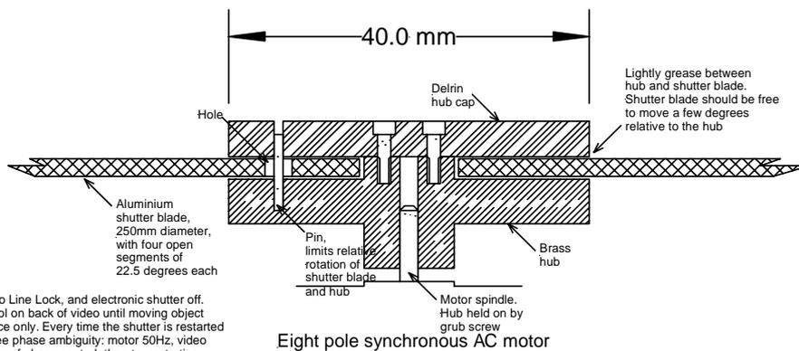
Set video camera to Line Lock, and electronic shutter off. Adjust phase control on back of video until moving object appears in one place only. Every time the shutter is restarted there is a 180degree phase ambiguity: motor 50Hz, video 25Hz. If out of range of phase control, then try restarting shutter.
