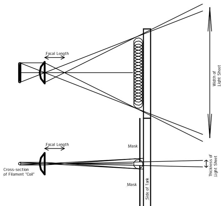
Figure 6: Sketch of optical arrangement for halogen lamp.
