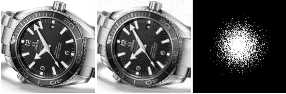
(a) 256 \times 256 full sampled (left) and 10% subsampled (center). Relative error to full sampling is 11.72%. Artefacts are obvious.
