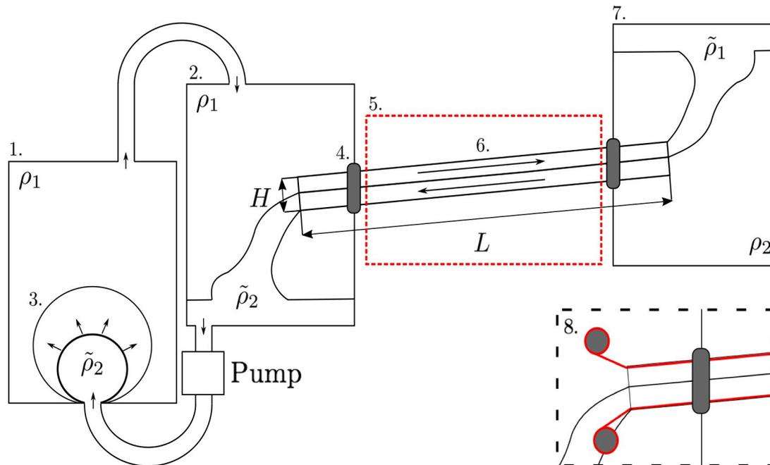
Allows moving boundaries, and ensures zero net flow
