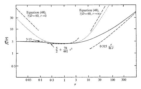
FIGURE 8. The shear-stress  $f_0^W$  is shown as a function of particle aspect ratio r by the continuous curve. The dashed curves are asymptotic forms. Schieraga's numerical results at  $\gamma/D = 60$  are shown by the dotted curve.
