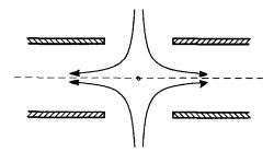
Fig. 1. Sketch of the opposed-jet device.
