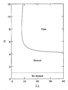
Fig. 5. Phase diagram showing the onset of pipe formation as a function of  $\hat{c}L$  and D.
