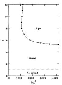
Fig. 10. Phase diagram of the formation of a pipe in planar flow as a function of  $\partial L^2$  and D with L = 100.
