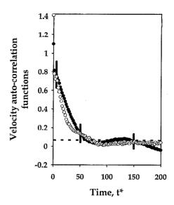
FIG. 6. Normalized velocity fluctuation autocorrelation functions for  $\phi$ =5% (a), 20% (b), and 40% (c). The solid circles are the experimental data for the vertical functions and the open circles for the horizontal functions. The uncertainty range is indicated for three data points on the vertical functions (the same uncertainty range is obtained for the horizontal functions).
