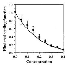
FIG. 3. Hindered settling function. The solid circles are the experimental data and the dotted curve corresponds to the Richardson-Zaki law with n=5.
