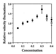
FIG. 4. The vertical relative velocity fluctuations,  $\sigma_{v\parallel}/\langle V_{\parallel}\rangle$ , vs  $\phi$ . The solid circles are the experimental data computed from the local velocities and the open circles from the extrapolated values of C(0).
