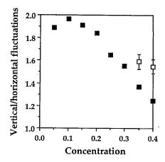
FIG. 5. The ratio between the vertical and horizontal standard deviations,  $\sigma_{v\parallel}/\sigma_{v\perp}$ , vs  $\phi$ . The solid squares are the experimental data computed from the local velocities and the open squares from the extrapolated values of C(0).
