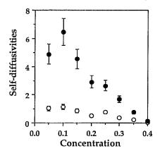
FIG. 10. The horizontal and vertical self-diffusivities made dimensionless by scaling with  $a\ V_S$  vs  $\phi$ . The solid circles are the experimental data for the vertical direction and the open circles for the horizontal direction.
