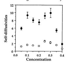
FIG. 11. The horizontal and vertical self-diffusivities made dimensionless by scaling with  $a\langle V_\parallel \rangle$  vs  $\phi$ . The solid circles are the experimental data for the vertical direction and the open circles for the horizontal direction.
