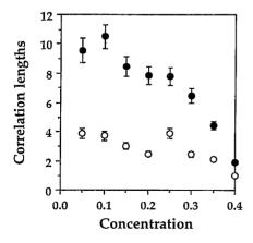
FIG. 7. The dimensionless horizontal and vertical correlation lengths,  $l_{c\perp}^*$  and  $l_c^*$ , vs  $\phi$ . The solid circles are the experimental data for the vertical direction and the open circles for the horizontal direction.
