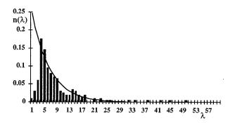
FIG. 1. Experimental results for the particle penetration depths for  $\theta_1$ =0.162±0.009 when particles were injected one by one with an upward flow.
