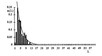
FIG. 3. Experimental results for the particle penetration depths for  $\theta_1=0.162\pm0.009$  when particles were injected one by one with no flow.
