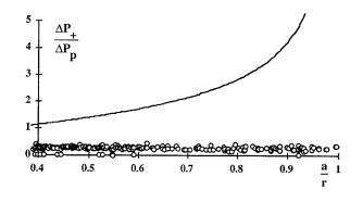
FIG. 6. Ratio between the extra-pressure in a tube due to a particle and the Poiseuille pressure drop (without a particle) for a tube in isolation (solid curve) and for a tube embedded in the network (empty circles).
