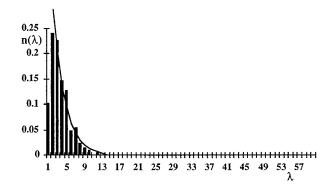
FIG. 4. Experimental results for the particle penetration depths for  $\theta_1=0.162\pm0.009$  when particles were injected by packets with no flow.
