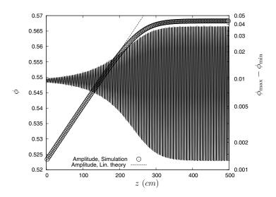
FIG. 3. Evolution of the disturbances towards a saturated state. The particle concentration is plotted with a heavy line, and the amplitude of the waves is plotted with circles. The linear theory prediction is plotted with dashed lines. Results plotted at t = 724.5s, obtained for f = 1.6Hz and  $\varepsilon_1 = 10^{-4}$ . The time step was  $\Delta t = 2 \cdot 10^{-4}s$ , space step was  $\Delta z = 4 \cdot 10^{-2}cm$ .
