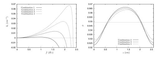
FIG. 7. Left. Growth rates for small amplitude disturbances. Right. Saturated waves profiles. Note that combination 1 in (5.1) and a frequency of 1.6Hz produces a stable mode. The horizontal dashed line indicates the homogeneous value  $\phi_o$ . Results on both plots were obtained with physical parameters as (4.5), with particle-phase pressure given by (4.8) and with coefficients as in (5.1).
