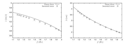
FIG. 11. Propagation velocity (right) and wavelength (right) of the saturated waves as a function of the frequency of the waves. In both plots,  $\phi_o = 0.549$  and all other parameters are as in (4.5).
