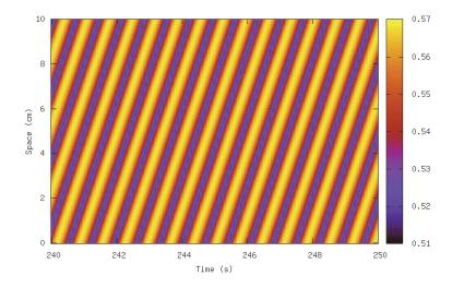
FIG. 4. Spatio-temporal plot of the steady-state waves for the simulation in Figure 3. The space value 0 corresponds roughly to z = 400cm.
