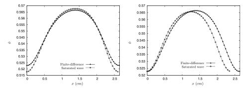
FIG. 13. Comparisons of the steady-state concentration profiles obtained via the unsteady finitedifferences simulations and via the saturated wave theory. On the left plot, both profiles were calculated for f = 1.6Hz. On the right plot, both profiles were calculated for the same  $\phi_{\min} = 0.52287$ . On both plots, physical parameters are given in (4.5).
