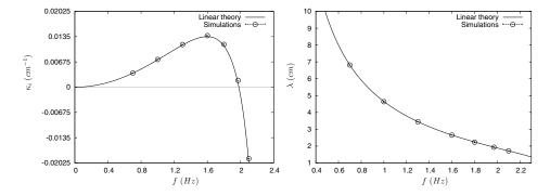
FIG. 2. Validation of the code for very small amplitude spatially evolving waves: spatial growth rates  $\kappa_i$  (left) and wavelength  $\lambda$  (right) of the waves. Results obtained for the parameters as in (4.5).
