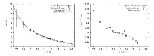
FIG. 14. Comparison of the wavelengths (left) and amplitudes (right) of the saturated waves obtained using via the unsteady finite-differences simulations and via the saturated wave theory with the experimental results available in [8]. The physical parameters given in (4.5).
