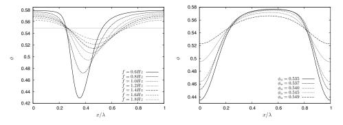
FIG. 5. Left. The influence of the frequency of excitation on the shape of the saturated waves. The horizontal dashed line indicates the homogeneous value  $\phi_o = 0.549$ . Right. The influence of the homogeneous concentration on the shape of the saturated waves. Results obtained for 1.6Hz. Results obtained for the parameters as in (4.5) and plotted against a normalized wavelength.
