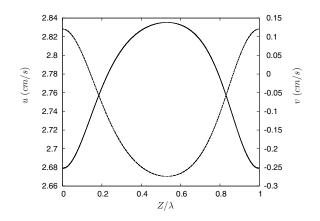
FIG. 12. Velocity profiles obtained for the configuration presented in (4.5) with  $\phi_o = 0.549$ . The propagation velocity of this wave is approximately c = 4.2 cm/s, and its frequency is f = 1.6 Hz. The continuous line denotes the particulate phase velocity, in phase with the concentration profile presented in Figure 8, and the dashed lines represent the out-of-phase fluid phase velocity.
