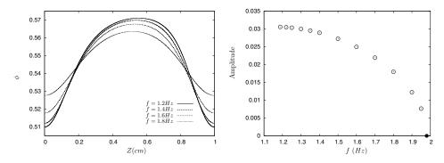
FIG. 10. Left. Comparison of the saturated wave profiles obtained for different frequencies. Right. Amplitudes of the waves as a function of the frequency. The black circle identifies the linear theory limit of zero amplitude. In both plots,  $\phi_o = 0.549$  and all other parameters as in (4.5).
