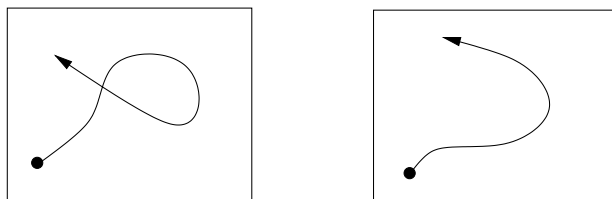
Figure 50: Motion in configuration space on the left, and in phase space on the right.
