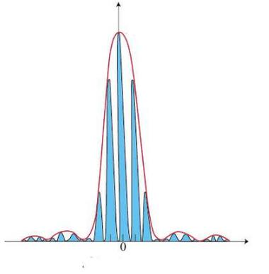
Figure 44: Double-slit diffraction pattern: plot of  $I$  against  $x$
