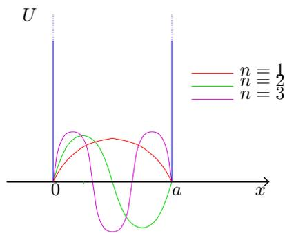
Figure 16: Lowest energy wavefunctions of the infinite square well.
