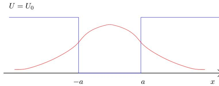
Figure 22: Groundstate probability density for the finite square well.
