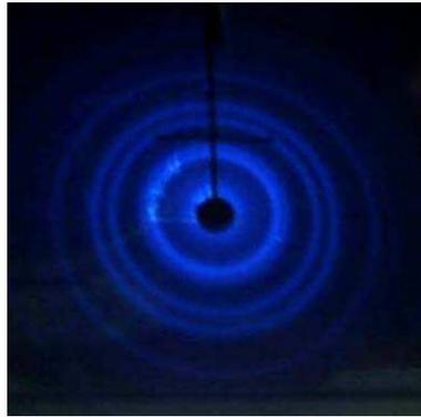
Figure 9: Electron diffraction from a crystal
