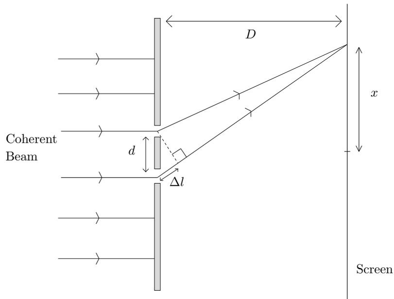
Figure 43: Double slit diffraction .
