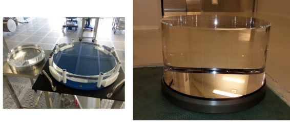
Figure 2.33. Advanced Virgo optics. Left: The power recycling substrate (35 cm in diameter, left) beside the beam splitter of 55 cm in diameter. Right: One of the Fabry–Perot cavity mirrors, which also serves as a test mass for the gravitational wave detector. Reproduced from [133], copyright IOP Publishing Ltd. All rights reserved.
