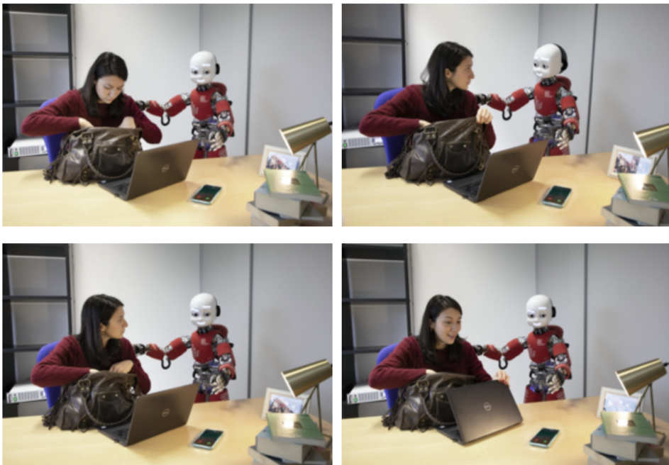
Figure 4.9. This sequence of pictures depicts a situation in which the iCub humanoid robot ( www.icub.org ) is interacting with a human, reading her intention to get her phone from her bag, and alerting her to the fact that it is on the desk, hidden from her by the laptop. This sequence has been staged to illustrate the future capabilities of a cognitive robot and has not yet been implemented. Reprinted from [223], copyright (2021) with permission by Springer Nature.
