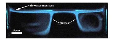
FIG. 1. Convective flow observed in a suspension of *Photobacterium phosphoreum*. The chamber is 6 cm long, 1 mm deep, and 1 cm high. Bacteria were cultured to a density of  $5.5 \times 10^8$  cells/cm<sup>3</sup> following the procedure detailed in the text. This image was acquired with a Nikon D300s equipped with a 60 mm f/2.8 macro lens, and an exposure time of 10 seconds.
