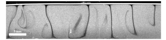
FIG. 5. Convection in a microsphere suspension. Darkfield image of the plumes observed in a suspension of 3  $\mu$ m diameter beads with 1% (w/w) salt concentration. The optical density was OD<sub>600 nm</sub> = 1 and the image was taken 30 minutes after the experiment had started.
