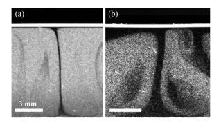
FIG. 8. Effect of microsphere size. (a) Plumes using 3  $\mu$ m diameter beads and (b) 6  $\mu$ m beads. The material, initial height, and salt concentration are the same in both cases. The optical density in both experiments is OD<sub>600 nm</sub> = 1 and the images were taken 45 minutes after the experiment had started.
