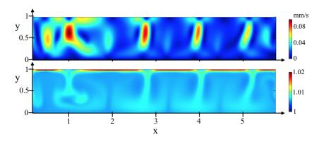
FIG. 15. Numerical results for 1% (w/w) initial salt concentration and 60 minutes after the experiment has started. Top: flow field; bottom: normalized salt concentration.
