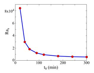
FIG. 13. Effects of varying  $t_0$ . Critical salinity number for a range of base-state waiting times  $t_0$ , with Pe = 0.2.
