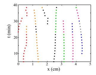
FIG. 6. Plume dynamics. Graphical representation of the plume position in time for an experiment using 3  $\mu$ m diameter beads and 1% (w/w) salt concentration. Different colors indicate the position of the first plume (red), second (orange), third (black), fourth (green), fifth (pink), sixth (blue), and seventh (grey).
