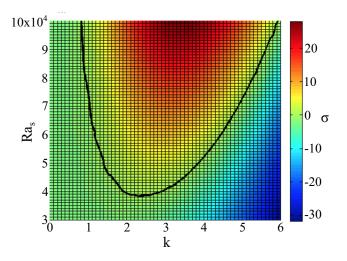
FIG. 10. Stability analysis. Values of the largest eigenvalue  $\sigma$  in the plane of salinity Rayleigh number Ra<sub>s</sub> and wave vector k. In black is the neutral stability curve. Parameters are those in Table II.
