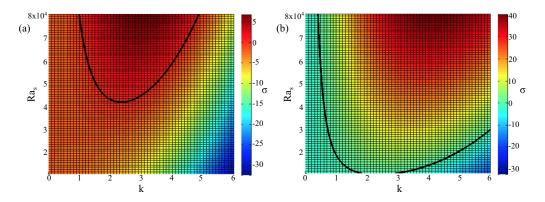
FIG. 11. Effect of Péclet number on the neutral stability curve. (a) Pe = 0.1 and Sc = 1, (b) Pe = 0.4 and Sc = 1.
