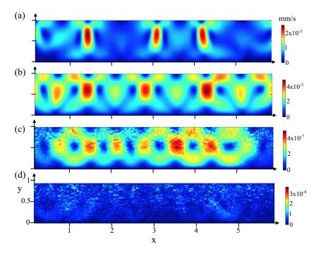
FIG. 16. Numerical flow fields for different initial salt concentrations. Snapshots at times corresponding to appearance of plumes for (a) 0.1% at t = 45 min., (b) 0.01% at t = 120 min, (c) 0.001% at t = 180 min, and (d) 0.0001% at 10 hours, at which point no plumes were observed.
