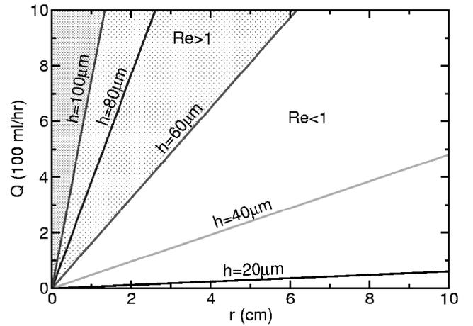
FIG. 3. Contour plot of fluid layer thickness  $h$  for various stalactite radii and fluid flow rates evaluated at  $\theta = \pi/2$ . At a thickness of  $60 \mu\text{m}$ , the Reynolds number approaches unity, and increases with increasing thickness. The shaded area beginning at a thickness of  $100 \mu\text{m}$  denotes the region in which diffusion time across the fluid layer is comparable to the time of the slowest relevant reaction.
