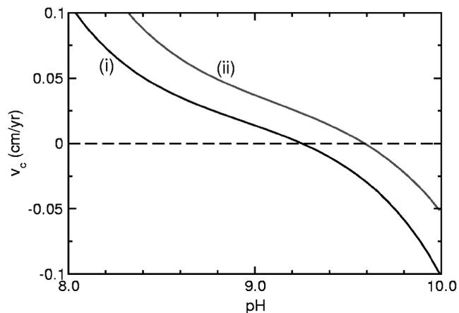
FIG. 6. Growth velocity  $v_c$  vs  $\text{pH}$ , using CO<sub>2</sub> partial pressure in the cave of  $3 \times 10^{-4}$  atm, a temperature of 20 °C, and (i)  $[\text{Ca}^{2+}]$  of 200 ppm and volumetric fluid flow  $Q=30$  cm<sup>3</sup>/h and (ii)  $[\text{Ca}^{2+}]$ =500 ppm and  $Q=5$  cm<sup>3</sup>/h. The formulas for the constants are taken from Ref. 4.
