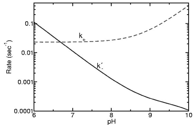
FIG. 4. Values for  $k_+$  and  $k'_-$  [Eq. (51)] as functions of pH are shown as dashed and solid lines, respectively. Note that  $k_+$  is much larger than  $k'_-$  at pH values typical of caves ( $\sim 9$ ), so  $[\text{Ca}^{2+}]$  must be significantly larger than  $[\text{CO}_2]$  for growth to occur.
