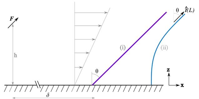
FIG. 5. Self-consistent model. An upstream point force  $\mathbf{F}$  parallel to the distal filament end produces shear flow that deflects the filament. Two variants: (i) rigid rod with a torsional spring at its base and (ii) a clamped elastic filament.
