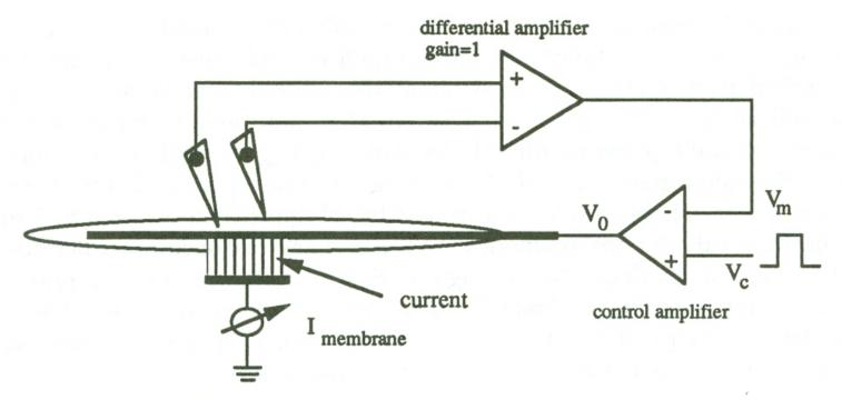
The *Voltage Clamp* is an electronic device which uses an applied current to maintain a chosen voltage across an excitable membrane while the conductance of the membrane goes throughh transient changes. This is done via feedback loop. A metallic electrode is inserted longitudinally down the centre of the axon. This short-circuits the inner axoplasmic core so that the interior is longitudinally isopotential and curren flow across the membrane is radial. This is called "space clamping".
