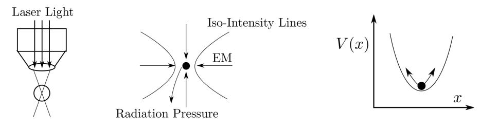
Assuming that the trapping potential is quadratic in lateral displacements x, the overdamped equation of motion of a microsphere in the trap is
