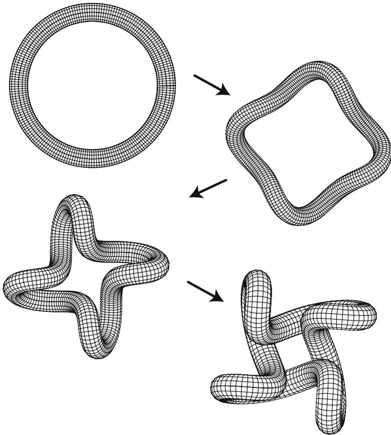
**Figure 6** Instability of the overtwisted ring. The twist is  $Tw = 30 \gg Tw_c$  and  $\alpha = 3/4$ , all modes between  $n = 2$  and  $n = 7$  are unstable and the fastest growing mode is  $n = 4$ .
