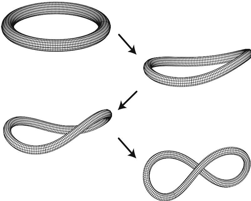
**Figure 2** Buckling of an unstable ring when the critical twist is first reached (twist not shown on the ring).
