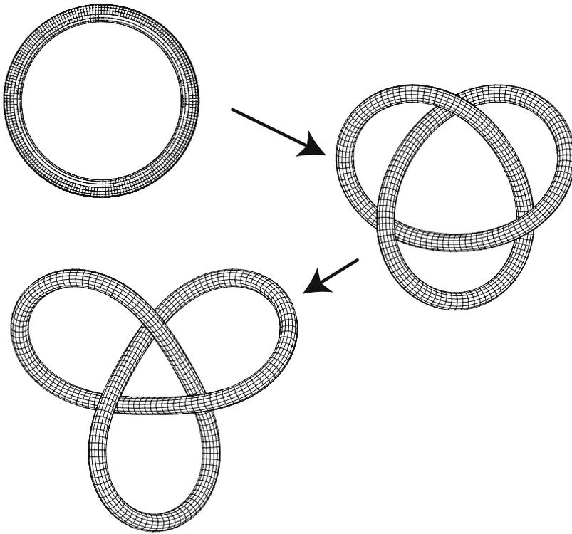
**Figure 5** Instability of a multicovered ring. Here  $p = 3, q = 2$  and the topology after unfolding is that of the trefoil knot.
