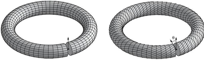
**Figure 1** Untwisted (left) and twisted ring (right). The total twist is given by the total angular rotation of an arrow pointing at any circle on the surface of the untwisted ring. Here the total twist is  $\frac{13}{2}\pi$ .
