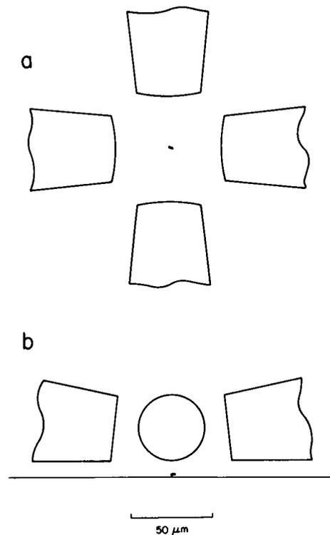
FIGURE 4 Tips of the tungsten wire microelectrodes. (a) top view; (b) side view. The tips were about  $40 \mu\text{m}$  across,  $70 \mu\text{m}$  apart (face to face), and  $10 \mu\text{m}$  away from the surface of the sapphire window. A tethered cell is shown to scale near the optical axis.
