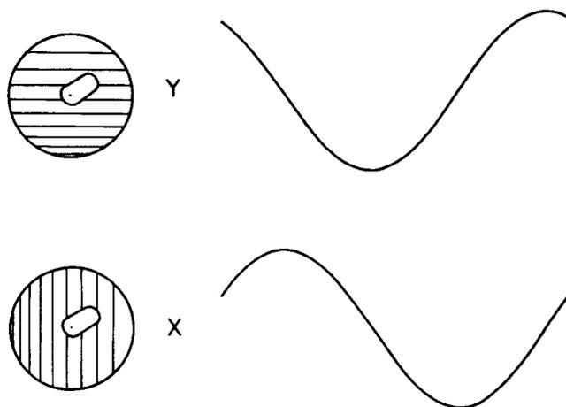
FIGURE 2 (Left)  $x$  and  $y$  linear-graded filters (4-mm diameter) viewed from above, showing the image of a tethered cell. The transmission of the  $x$  filter increases linearly from left to right, and the transmission of the  $y$  filter increases linearly from bottom to top (both from 16% to 89%). (Right) intensity of transmitted light obtained when the image rotates at a constant speed one revolution clockwise.
