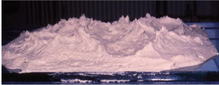
**Fig. 1.** One of the two failure surfaces obtained by separating two 30 cm  $\times$  30 cm glass plates between which a 2 cm thick granular adhesive paste was confined (paste  $P_\beta$ , sect. 2.1) (from [19], with permission).
