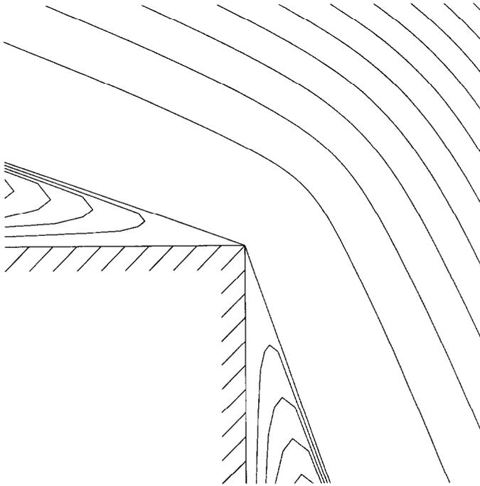
Fig. 4. Streamlines for the aligned flow at  $\phi = 180$ . The increments between the bulk streamlines are 1000 times the increments between the recirculating streamlines.
