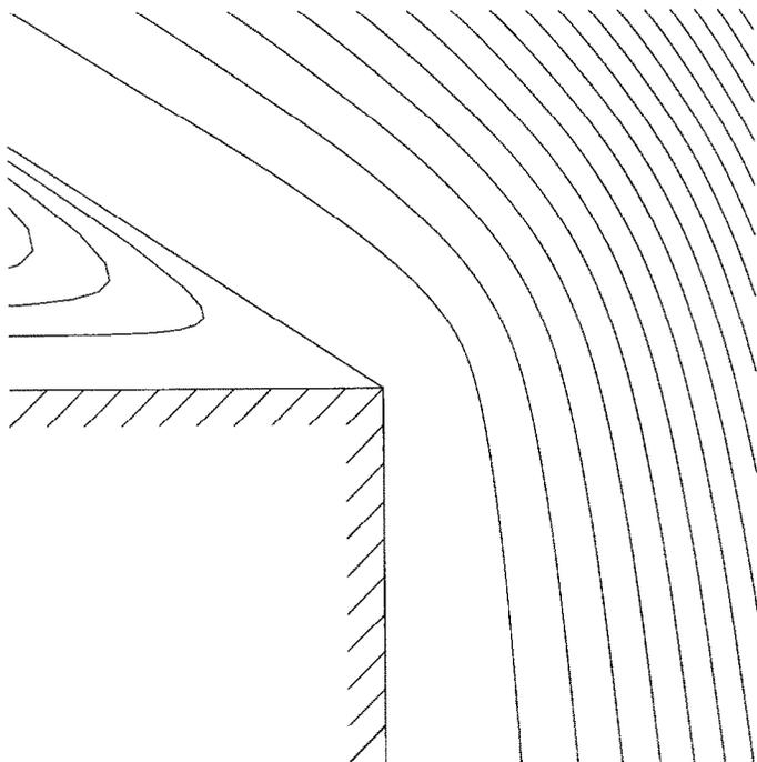
Fig. 8. Streamlines for the asymmetric de-aligned flow at  $\phi = 32$ . Increments between the bulk streamlines are 20 times the increments between the recirculating streamlines.
