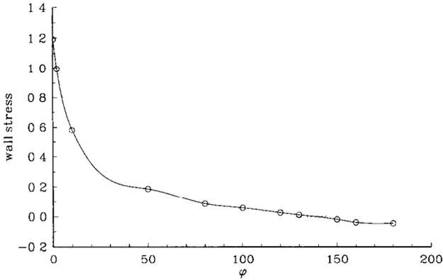
Fig. 3. The wall shear rate,  $f''(\frac{3}{4}\pi)$ , for the aligned solutions as a function of  $\phi$ .
