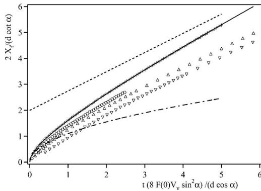
FIG. 13. Variation of the normalized front distance to the origin  $2X_f/(d \cot \alpha)$  as a function of the normalized time  $t(8k_v V_v \sin^2 \alpha)/(d \cos \alpha)$ . (+) Numerical data. Continuous line: fitted variation using Eq. (29). Experimental points ( $\circ$ ):  $\alpha=1^\circ$ , ( $\triangle$ )  $\alpha=2^\circ$ , ( $\nabla$ )  $\alpha=3^\circ$ . Dash-dotted line: diffusive spreading at early times. Dotted line: limiting constant velocity motion at very long times.
