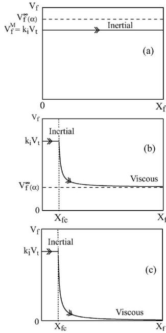
FIG. 5. Front velocity variation as a function of distance  $X_f$  from the gate valve (continuous line). (a)  $\alpha \neq 0^\circ$ :  $k_i V_t \leq k_v V_v \sin \alpha$ . (b)  $\alpha \neq 0^\circ$ :  $k_i V_t > k_v V_v \sin \alpha$ . (c)  $\alpha = 0^\circ$ . Dashed line:  $k_v V_v \sin \alpha$ . Dotted line:  $X_f = X_{fc}$ . Arrows: trend of the evolution of the velocity with time.
