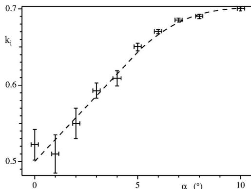
FIG. 8. Variation of the coefficient  $k_i$  characterizing the front velocity in the inertial regime as a function of the tilt angle  $\alpha$  ( $At=3.9 \times 10^{-3}$ ,  $d=20$  mm,  $\nu=10^{-6}$  m<sup>2</sup>/s). The dashed line is a guide for the eye; horizontal and vertical lines on the data points indicate the error bars.
