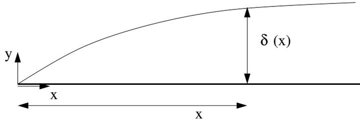
With no  $x$ -length scale imposed in the definition of the problem, we take  $L = x$  itself, so heading for a similarity solution. The estimate of the boundary layer thickness of §7.3 gives
