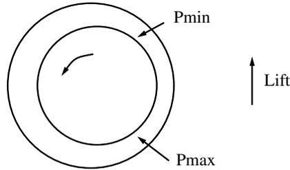
where the pressure variation ensures a constant flux around the bearing.
