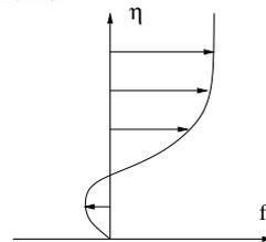
The solutions with reverse flow are probably unstable and impossible to set up in an experiment. The two branches come together at  $m = -0.0904$ , corresponding to a wedge angle of  $180^\circ + 18^\circ$ .
