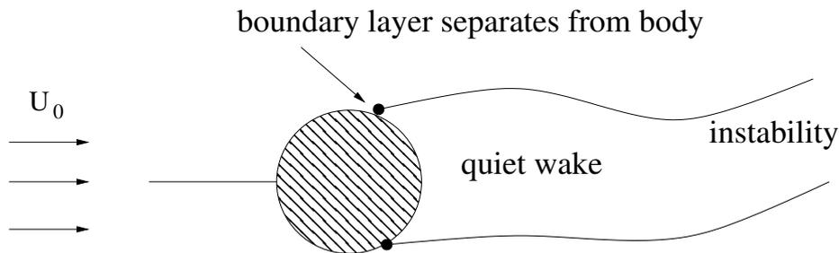
The separation point is roughly at  $\theta = 80^\circ$  when laminar at  $Re = 10^{5-}$ , but moves to  $120^\circ$  at  $Re = 10^{5+}$  when the flow becomes turbulent. The turbulence reduces the cross-section of the wake, which thus reduces the drag, so trip-wires are used to trigger turbulence at lower  $Re$ .
