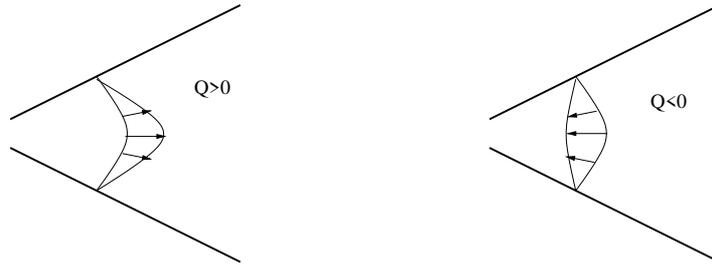
At high Reynolds numbers with in flow  $Q < 0$ , there is away from the walls (Euler limit) a uniform potential flow  $u_r = -|Q|/2\alpha r$ . Near the walls there are boundary layers. These boundary layers are governed by
