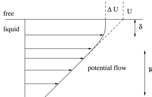
The tangential stress in the potential flow  $\mu U/R$  is corrected by  $+\mu \Delta U/\delta$  to go to zero on the boundary. Hence
