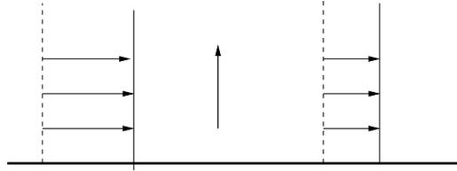
mass conservation gives an advection away from the wall. With advection and diffusion away from the wall, it is not possible to confine the vorticity near to the wall, so the boundary layer structure breaks down. Typically the boundary layer separates from the wall and head off in the interior of the flow.
