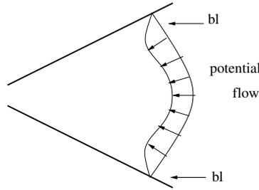
At high Reynolds numbers with out flow  $Q > 0$ , a central jet develops at moderate  $Re$ , with reverse flow near the walls as  $Re$  increases.
