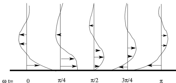
The figure shows a 'propagation': the plate drags the fluid, the fluid above starts to move and through inertia continues to move after the plate has stopped. Note activity in the second wavelength is very very small,  $e^{-2\pi} \approx 10^{-3}$ .
