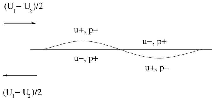
The crowding of the streamlines over the peaks, increases the flow, with a corresponding decrease in the troughs. The need to accelerate to the peak and decelerate after requires a pressure minimum on the peak – Bernoulli. Similarly there is a pressure maximum in the troughs.
