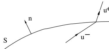
i.e. the normal component of velocity must be continuous across  $S$ . [Not so at an evaporating interface where  $\rho$  would jump.] In particular, at a fixed boundary,  $\mathbf{u} \cdot \mathbf{n} = 0$ . And if the moving boundary of a fluid is given by  $F(\mathbf{x}, t) = 0$ , then since the surface consists of material points:
