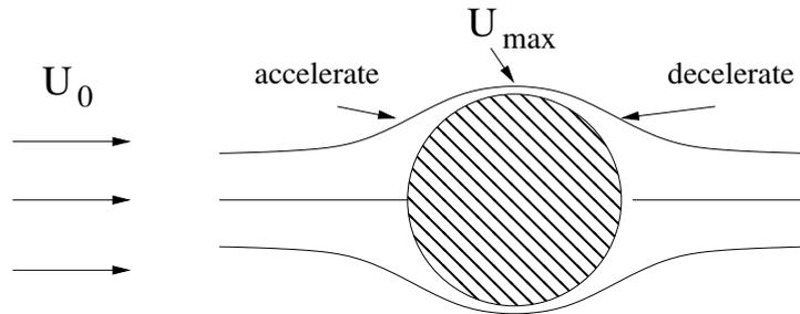
The potential flow past the body has a maximum and afterwards decelerates. If one uses this potential flow as the external flow  $U(x) \propto \sin \theta$  in the boundary layer equations, one finds that the solution blows up at  $\theta = 104.5^\circ$ . One observes in experiments
