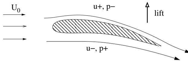
A clockwise circulation makes the flow faster along the top surface than along the bottom. By Bernoulli (in the potential flow) the pressure is lower on the top surface than on the bottom surface. Hence there is an upward lift force.
