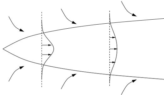
The Reynolds number  $Re = U\delta/\nu \propto x^{1/3}$  increases, so at large  $x$  the jet becomes unstable. One can also solve the axisymmetric “round” jet, momentum wakes behind towed objects, momentum-free wakes behind self-propelled objects, and shear layers.
