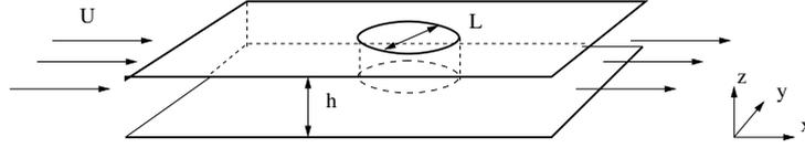
Flow is in the thin gap of thickness  $h$  between two fixed plates, with obstacles of size  $L$ . If  $h \ll L$ , the flow is mostly in  $xy$ -plane. The no-slip boundary condition is  $\mathbf{u} = 0$  on  $z = 0$  and  $z = h$ . Then
