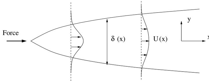
We need to find the scalings of the thickness of the jet  $\delta(x)$  and the centre line velocity  $U(x)$ . Balancing the inertial and viscous terms in the boundary layer equations
