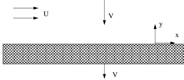
Far from the wall, there is a cross-flow  $U$  and the suction  $V$ . We take  $\mathbf{F} = 0$  and  $\nabla p = 0$ . We try a flow field  $\mathbf{u} = (u(y), -V, 0)$  with  $u \rightarrow U$  as  $y \rightarrow \infty$ , and no-slip  $u = 0$  on  $y = 0$ .
