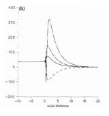
Continuous curve is correct solution. Others have spurious oscillations.
