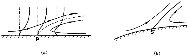
Figure 5.7 Zero stress and separation: (a) velocity profiles and streamlines \psi_p = \text{const.} near a point of zero stress (b) streamlines \psi_E = \text{const.} near a separation point S
