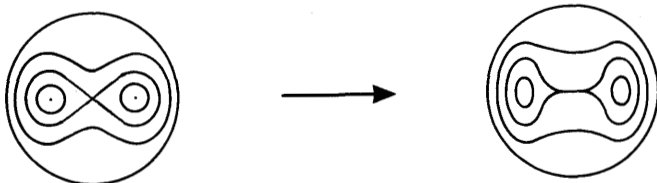
Fig. 6. Relaxation of field with two elliptic neutral points and one hyperbolic point: a current sheet discontinuity forms with a cusped structure at its end-points (K. Bajer 1986).
