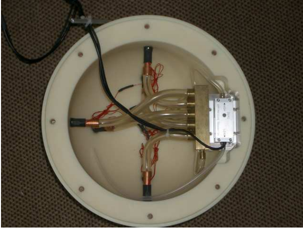
Figure 2. Internal view of pressure sensor. Eight outlets are connected through a junction and moisture trap to a single differential transducer. The other of the transducer is connected to a chamber in the stalk that provides a constant reference pressure.
