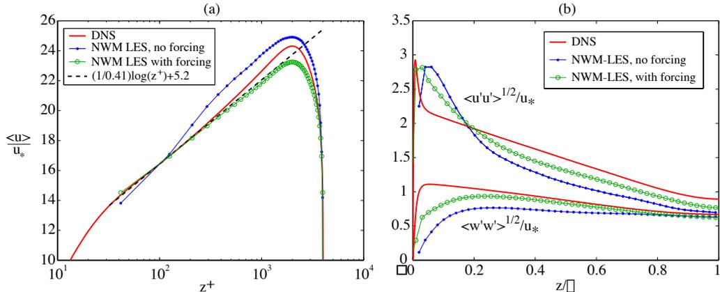
Figure 2. (a) Mean velocity profiles and (b) streamwise and wall-normal  $rms$  velocity for smooth wall channel flow with  $Re_* = 2000$
