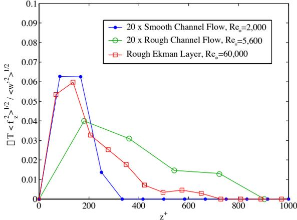
Figure 1. *r.m.s.* of the stochastic forcing function with the amplitude evaluated dynamically for  $z/\delta < \Delta_f$ . Note that the channel flow cases have been scaled by a factor of 20.
