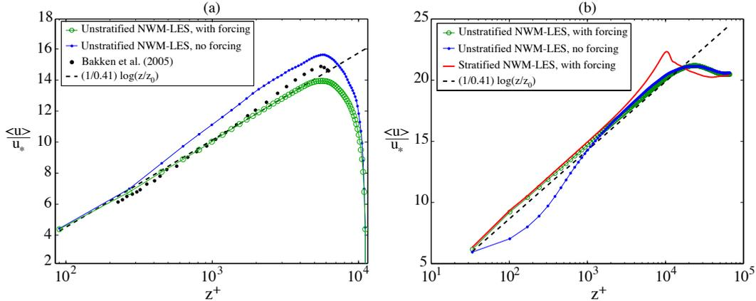
Figure 3. (a) Mean velocity profiles for rough wall channel flow with  $z_0/\delta = 2.81 \times 10^{-3}$  and  $Re_* = 5600$ , (b) Mean velocity profiles for a bottom Ekman layer with  $z_0/\delta = 5.7 \times 10^{-5}$  and  $Re_* = 60,000$ .
