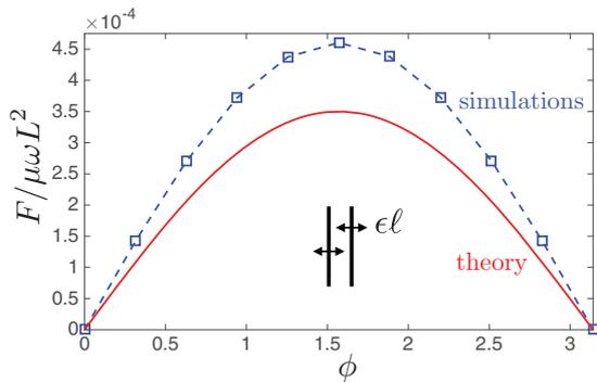
Fig. 3: (Colour online) Net force induced on the fluid by a two-rod pump,  $F/\mu\omega L^2$ , as a function of the phase difference,  $\phi$ , between the rods. Dashed line and symbols: slender-body theory simulations; Solid line: theory (eq. (31)). The dimensionless distance between the rods is  $h/L = 0.1$ , their aspect ratio  $a/L = 0.025$  (so that  $a/h = 0.25$ ) and the motion amplitude is  $\epsilon\ell = h/10$ .
