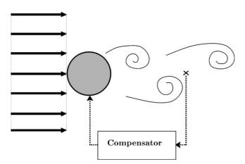
Fig. 1. Vortex shedding control approximately modeled by the idealized 1D system: based on noisy measurements downstream of the cylinder, the compensator constructs a state estimate which, in turn, is used to compute control feedback applied at the cylinder itself.
