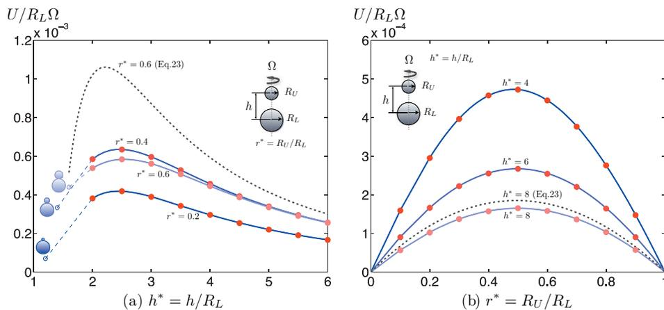
FIG. 4. Propulsion speed of a separated snowman as a function of (a) the separation distance, and (b) ratio of the radii, at  $De = 0.1$  and  $\zeta = 0.5$ . Red dots: numerical results in an Odroyd-B fluid. Blue solid line: second-order fluid analytical calculation. Black dotted line: simplified model (Eq. (50)).
