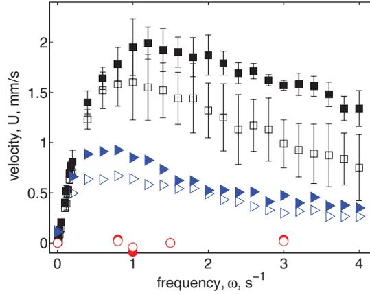
FIG. 4. Mean forward swimming speed,  $U$  (mm/s), as a function of the oscillating frequency,  $\omega$  (Hz). Filled and empty symbols correspond to Boger and Newtonian fluids, respectively.  $\square$  (black): fluids N2 and B2, flexible swimmer;  $\triangleright$  (blue): fluids N1 and B1, flexible swimmer;  $\circ$  (red): fluids N1 and B1, rigid tail swimmer. The error bars depict the standard deviation of the measurements for the N2 and B2 fluids which were repeated four times.
