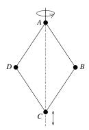
Identify suitable generalized coordinate(s) and write down the Lagrangian of the system.
