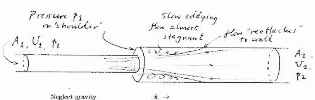
Immediately downstream of the junction, there is a complicated eddying behaviour. Ultimately the flow reattaches to the boundary and there is an approximately uniform flow far downstream.
