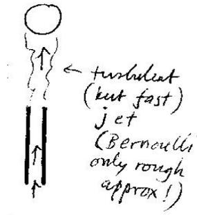
Bernoulli helps understand stability to sideways displacement. The flow past the ball is faster on the side nearest the pipe axis.
