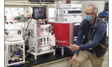
Figure 1. A continuous flow reactor at Argonne National Laboratory’s Materials Engineering Research Facility uses the optimization solver ParMOG to perform autonomous discovery [2].
