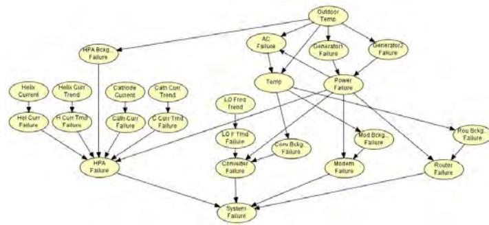
**Figure 3. Bayesian network for failure prediction and diagnosis for a satellite earth terminal.**
