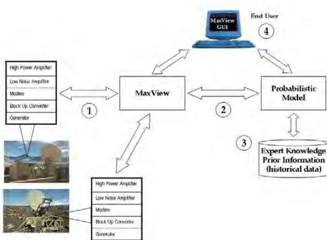
**Figure 4. Interface between MaxView monitoring and control software and the Bayesian network.**
