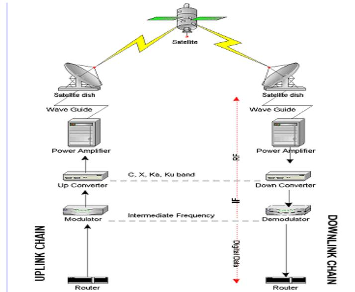
**Figure 1. Basic components of a satellite earth terminal link.**
