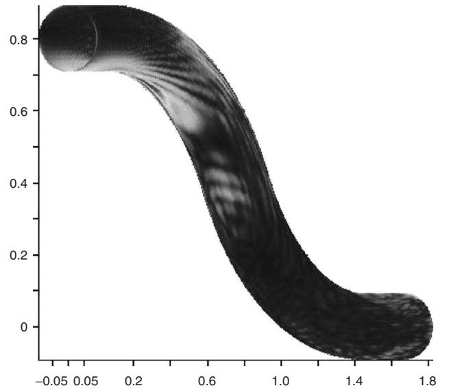
Fig. 1 Surface current amplitudes on waveguide of length 220 and diameter 20 wavelengths
