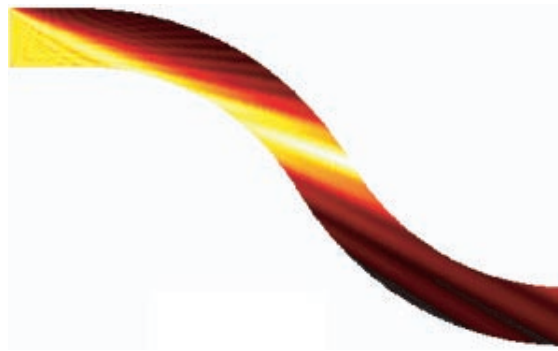
Figure 3. Amplitude of the incident field using Kirchoff integral over aperture, i.e. the aperture field, inside a waveguide of diameter 20\lambda' over a length of 200\lambda , for the field incident at -20^\circ .
