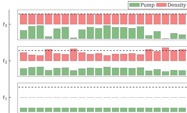
FIG. 1: The schematics of operation of the GD simulator. Initially, at t = t_1 all CCs are equally pumped (green bars) below the threshold, and all have negligible densities. As the pumping intensities increase and depending on the connectivity between CCs, the different densities emerge (red bars) as shown at some t = t_2 . The individual control of the pumping intensity as described by Eq. (6) leads to the steady state with all the densities reaching the threshold at t = t_3 .
