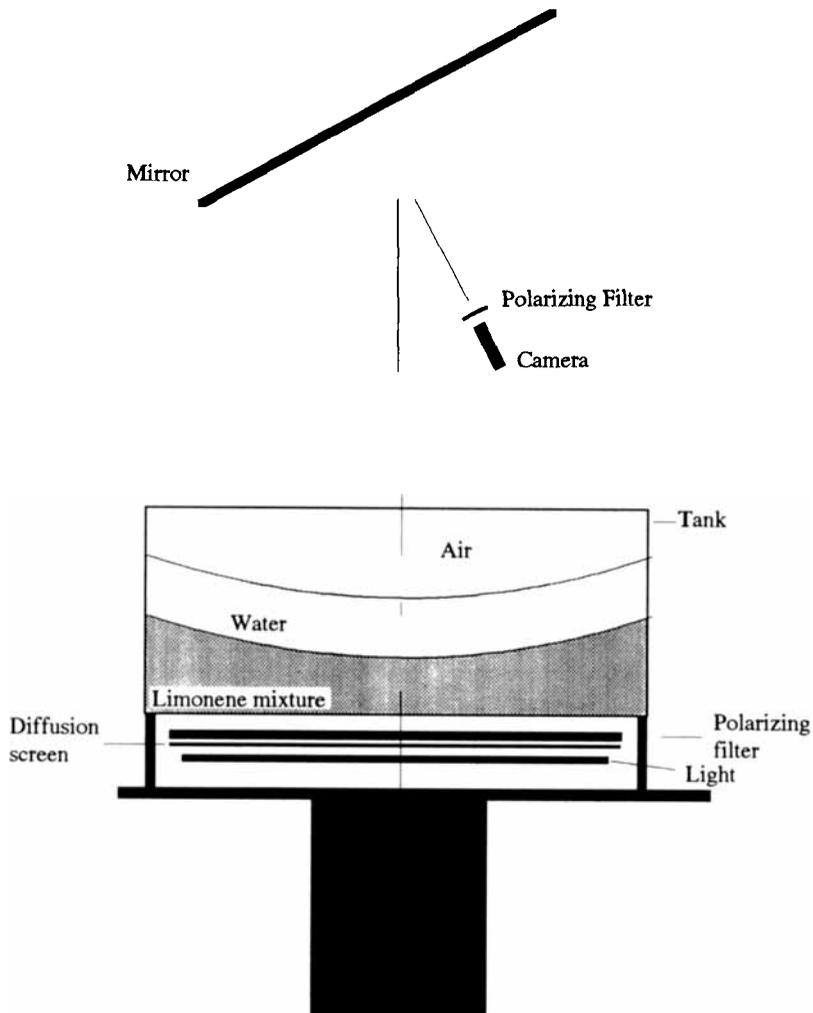
Figure 3 A schematic of experimental equipment.
