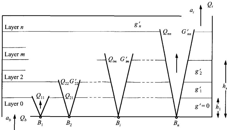
FIGURE 4. Ventilated enclosure with  $n$  positive buoyancy sources.
