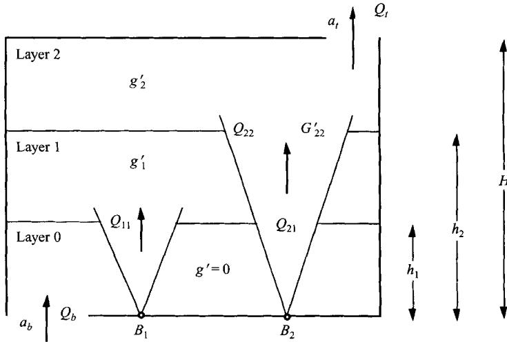
FIGURE 1. Ventilated enclosure with two positive buoyancy sources.
