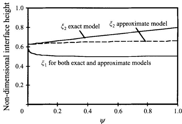
FIGURE 2. Comparison of the exact and approximate theoretical predictions of the non-dimensional interface heights  $\xi_1$  and  $\xi_2$  as functions of the ratio  $\psi = B_1/B_2$  of the buoyancy fluxes, for the dimensionless vent area  $A^*/H^2 = 0.0167$ . The solid curves are the exact solutions given by Cooper & Linden (1996) neglecting entrainment flux  $Q^*$  and the dashed curves are the approximate model discussed in §2.
