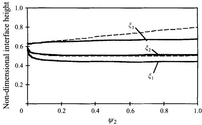
FIGURE 5. Dimensionless interface heights  $\xi_1$ ,  $\xi_2$  and  $\xi_3$  (solid curves), for the approximate solution for three plumes with  $B_1 = \frac{1}{2}B_2$ , plotted against the buoyancy flux ratio  $B_2/B_3$ . The dashed curves are the two-plume solution for the same dimensionless vent area  $A^*/H^2 = 0.0167$ .
