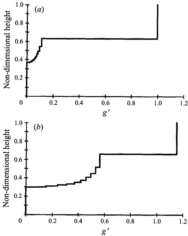
FIGURE 9. The stratification produced by  $n = 10$  plumes, with strengths given by the arithmetic progression, plotted against the dimensionless height  $Z$  within the enclosure. The strength  $B$  of the strongest plume is 20 kW, the dimensionless vent area  $A^*/H^2 = 0.0167$  and  $H = 5$  m. In (a)  $\beta = 0.01$ , and in (b)  $\beta = 0.1$ . Note that  $g' = 1 \text{ m s}^{-2}$  corresponds to a temperature difference of about 30 °C.
