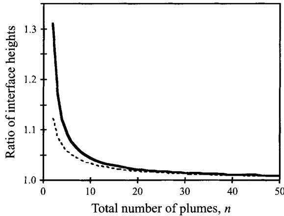
FIGURE 8. The ratio of interface heights  $\xi_2/\xi_1$  plotted against  $n$  for the case of  $(n-1)$  equal plumes of strength  $B_i = B$ , and one strong plume of strength  $B_n$ , such that  $\psi_i = B/B_n \ll 1, i = 1, \dots, n-1$ . The dashed curve is for  $\psi = 0.01$ , and the solid curve is for  $\psi = 0.5$ .
