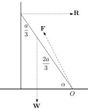
The normal reaction of the ground on the foot of the ladder and the frictional force acting on the foot of the ladder are combined into a single (unknown) force  $\mathbf{F}$ , acting in an unknown direction. There is no friction at the upper end of the ladder because the wall is smooth.
