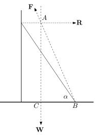
Note first that the three lines of action must intersect. Otherwise, we could take moments about the point of intersection of any pair (if not parallel); the two corresponding forces would have no moment about this point, since their lines of action passes through the point, leaving a non-zero moment from the third force. The total moment would thus be non-zero and the rod could not be in equilibrium.
