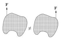
In general, each force acting on a body can be thought of as having two effects: a tendency to translate the body in the direction parallel to the line of action of the force; and a tendency to rotate the body.<sup>1</sup> Clearly, for the body to be in equilibrium these effects must separately balance.
