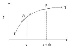
Look at **vibrating string**. Let the string be under tension T with mass per unit length  $\rho$ . The displacement at position x and time t is y(x, t). Consider element AB of length dx.
