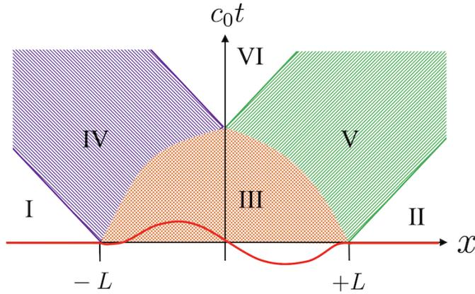
**Figure 25.** An initial disturbance in a region  $|x| < L$  propagates to the left and to the right. Regions I,II and VI are undisturbed; regions IV and V have only left-moving and right-moving waves respectively, and anything can happen in region III.
