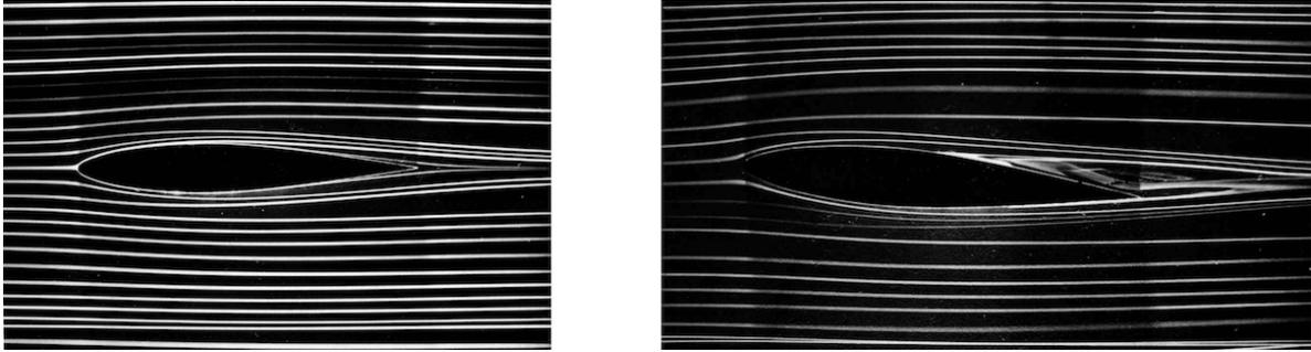
**Figure 14.** The flow, from left to right, around a streamlined object at  $Re \approx 7000$ . On the left, the object is aligned with the streamlines and the boundary layer merges smoothly into the flow at the trailing edge. On the right, the object is inclined by  $5^\circ$ . The boundary layer separates from the object on the upper edge.
