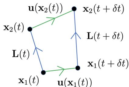
$$\begin{aligned} \mathbf{L}(t + \delta t) &\approx \mathbf{x}_2(t + \delta t) - \mathbf{x}_1(t + \delta t) \\ &\approx \mathbf{L}(t) + (\mathbf{u}(\mathbf{x}_2(t)) - \mathbf{u}(\mathbf{x}_1(t))) \delta t \end{aligned}$$
