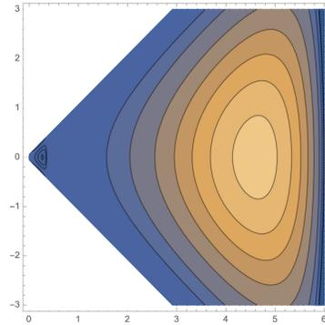
The stream function for a right-angle corner is shown in the figure, clearly exhibiting one such eddy. The logarithm means that both the size of the eddies, and the amplitude of the stream function, vary exponentially. The centres of consecutive eddies lie at
