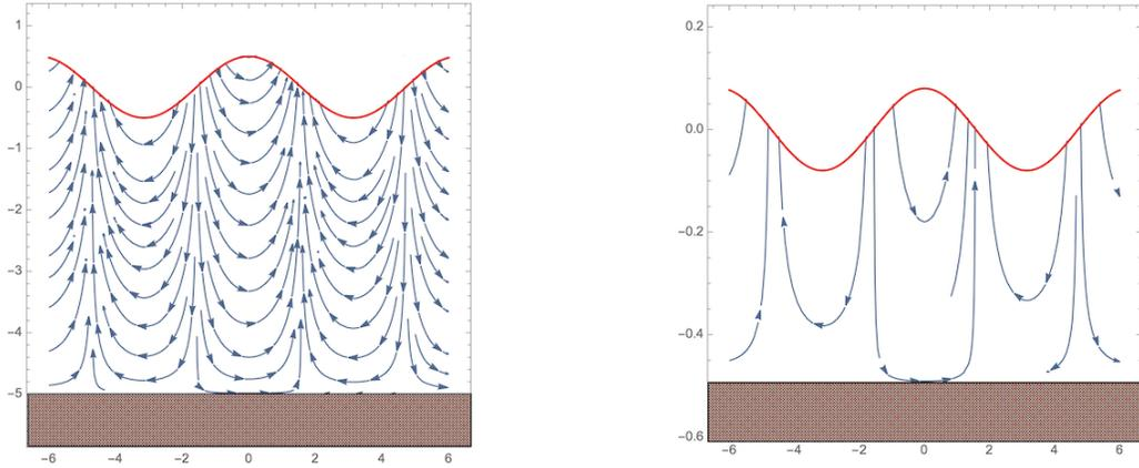
**Figure 21.** The velocity field for deep water waves on the left, with  $kH = 5$ , and shallow water on the right with  $kH = 0.5$ . (Note the different scales on the vertical axes!) The streamplot shows only the direction of the velocity field, not its size. In deep water, the velocity is exponentially smaller at the bottom than the top.
