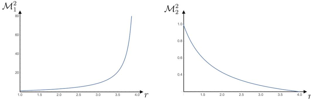
**Figure 29.** The initial and final Mach numbers as a function of the compression ratio  $r$ , plotted for  $\gamma = 5/3$ . We have  $\mathcal{M}_1 \geq 1$  and  $\mathcal{M}_2 \leq 1$  for all values of  $r$ .
