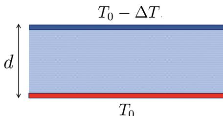
$$T = T_0 - \Delta T \frac{z}{d} \quad \text{and} \quad P = P_0 - \rho_0 g \left( z + \frac{\alpha \Delta T}{2d} z^2 \right) \quad (5.23)$$
