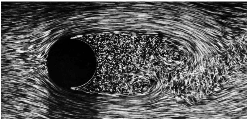
**Figure 16.** A flow around the circular cylinder, now with  $Re \approx 2000$ . We're now at values where the boundary layer theory should work. The picture clearly shows laminar flow at the front of the cylinder, where the boundary layer remains attached. It separates somewhere near the top and bottom of the cylinder, leaving a turbulent wake.
