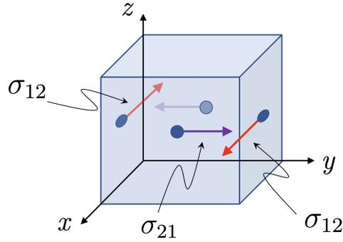
**Figure 9.** The torque experienced by a small parcel of fluid. The red arrows depict  $\sigma_{12}$ , the purple arrows  $\sigma_{21}$ . (The purple arrow on the furthest face is unlabelled to avoid clutter.)
