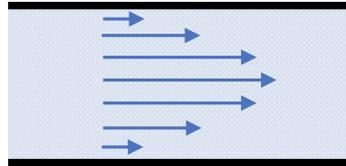
This is known as *Poiseuille flow*. The minus sign is sensible: it tells us that if the pressure is greatest to the left, so  $dP/dx < 0$ , then the fluid moves to the right. Clearly the speed increases as we move away from the edges and is maximum in the middle where  $z = 0$ . Again, the flow has vorticity induced by the no-slip boundary condition.
