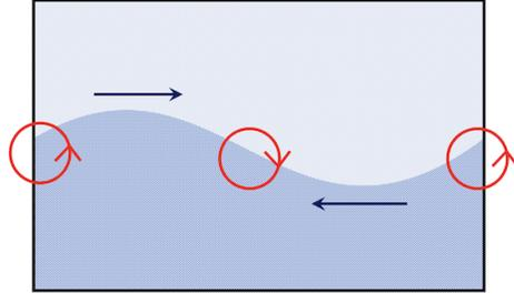
no change to the vorticity at the maxima and minima, but the vorticity alternates clockwise/anti-clockwise at the midway points of the perturbation, as shown in the figure. This acts to push the crests up, and the troughs down, again
