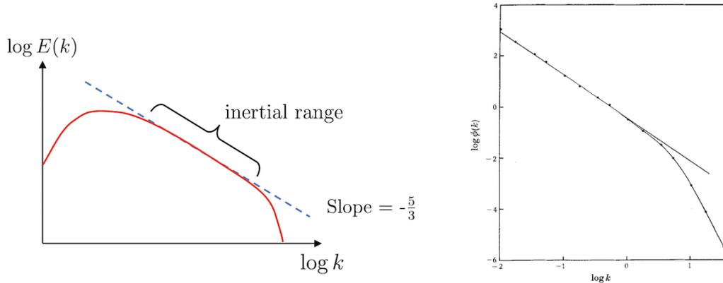
**Figure 35.** On the left, a sketch of the expected behaviour of  $E(k)$  based on dimensional analysis. The energy is injected at small  $k$  and dissipated at large  $k$ , with the characteristic  $E(k) \sim k^{-5/3}$  in the inertial range. On the right, data.
