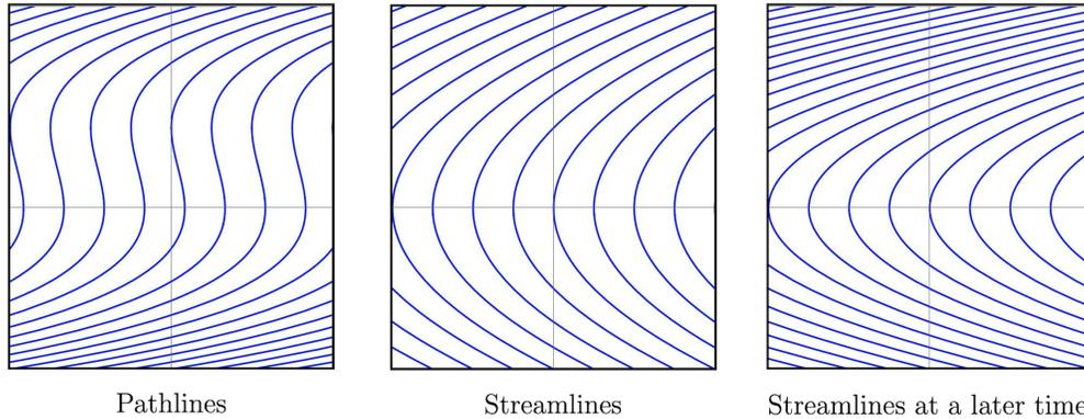
**Figure 1.** The pathlines for particles in the flow  $\mathbf{u} = (yt, 1)$  are shown on the the left. These are a history of the flow. The middle and right hand figures show streamlines, with the right-hand figure at a later time.
