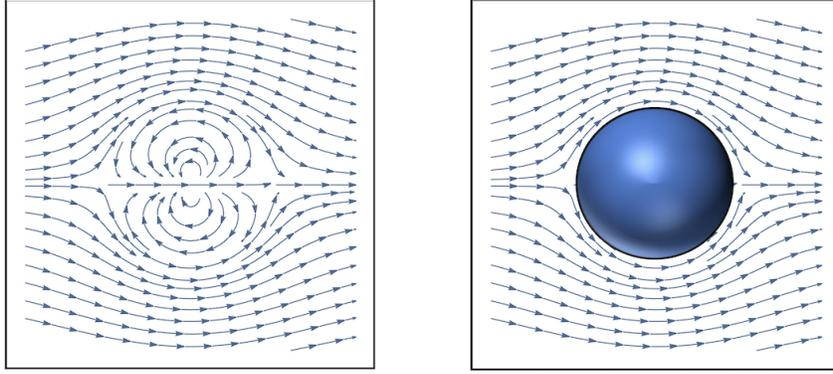
**Figure 10.** Stokes flow around a sphere. The left-hand figure shows the flow in the middle is in the opposite direction to the flow outside. This means that it must vanish on some surface. This surface is that of the solid sphere, as shown on the right.
