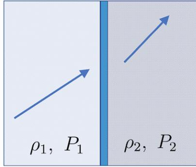
**Figure 28.** Two flows separated by a shock wave.
