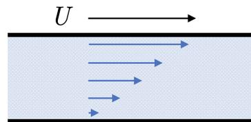
The result is known as *Couette flow* and is shown in the figure. Flows of this kind, in which adjacent layers of fluids move at different speeds, are collectively referred to as *shear flows*.
