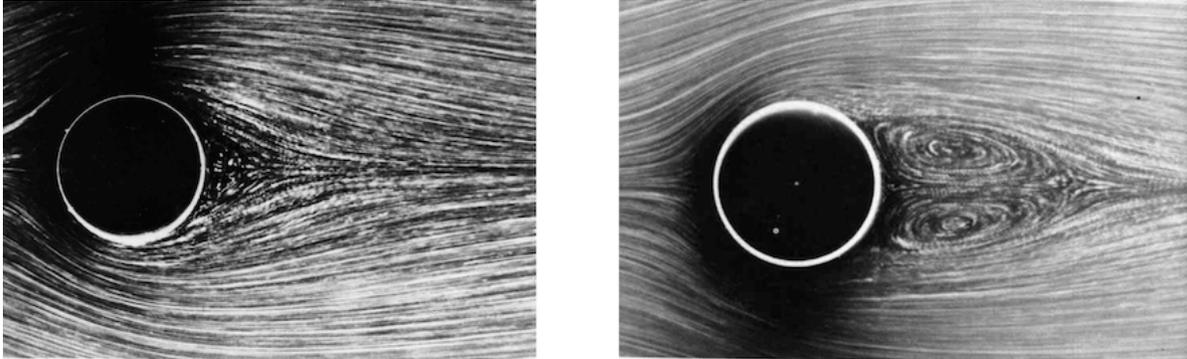
**Figure 15.** The flow around a circular cylinder with  $Re \approx 10$  on the left, and  $Re \approx 26$  on the right. In both cases, the flow separates from the cylinder at some point, leaving two trailing eddies in the wake (more visible in the second picture).
