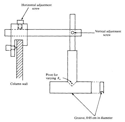
FIGURE 5. The particle release mechanism. Not drawn to scale.
