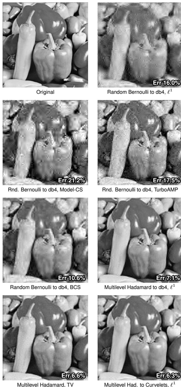
Fig. 11. Compressive Imaging (CI) example: 12.5% subsampling at  $256 \times 256$ . The multilevel subsample map is the one from Fig. 2.
