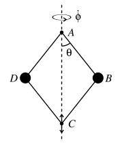
[This is a model of a *centrifugal governor* - a device that in the past has been used to regulate the speed of engines, in particular steam engines.]
