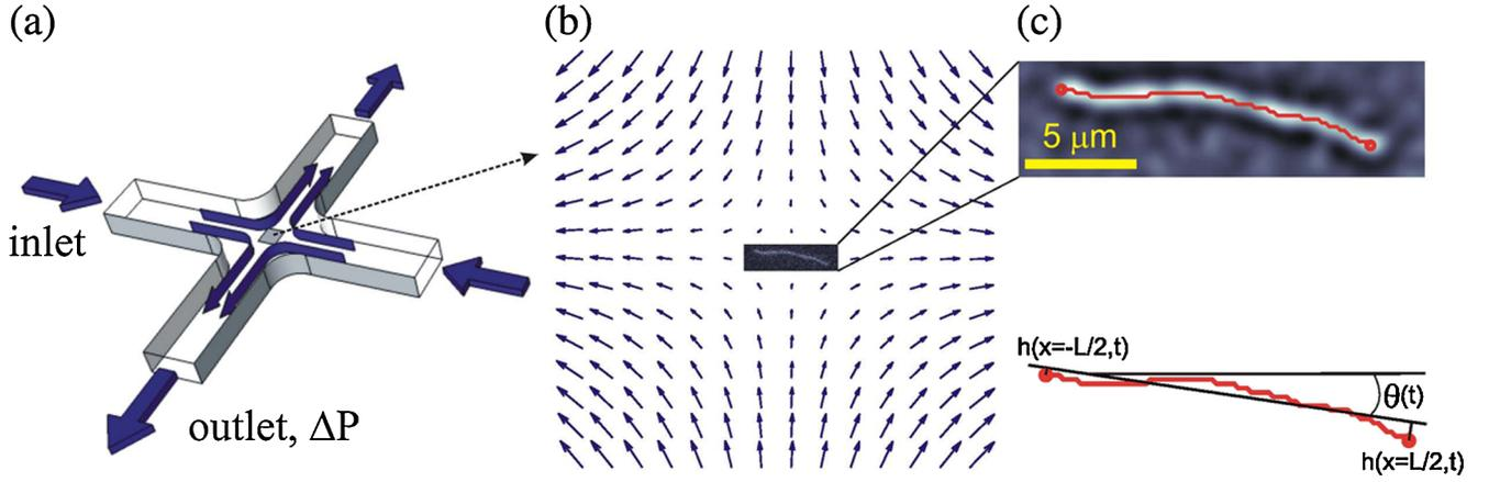
FIG. 1 (color online). Experimental setup. (a) Microfluidic cross-flow geometry controlled by a pressure difference  $\Delta P$  between inlet and outlet branches. (b) Close-up of the velocity field near the stagnation point, showing a typical actin filament. (c) Raw contour (red) of an actin filament and definition of geometric quantities used in the analysis.
