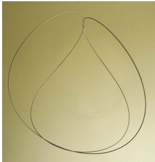
Figure 1. Minimum-energy configuration of a stiff wire in the form of a figure-of-eight knot; the two points of double contact are evident.
