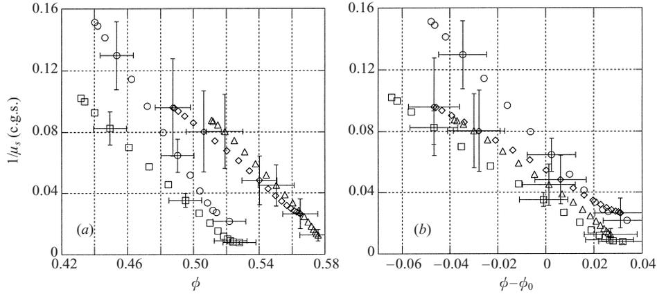
FIGURE 18. Influence of the bed to particle ratio  $D/d_s$  on  $\mu_s$ . (a)  $1/\mu_s$  plotted against  $\phi$ ; (b)  $1/\mu_s$  plotted against  $\phi - \phi_0$ .  $\circ$ ,  $\phi_0 = 0.488$ ;  $\square$ ,  $\phi_0 = 0.496$ : combination 7 with  $D/d_s \approx 10$ .  $\triangle$ ,  $\phi_0 = 0.549$ ;  $\diamond$ ,  $\phi_0 = 0.534$ : combination 6 with  $D/d_s \approx 25$ .
