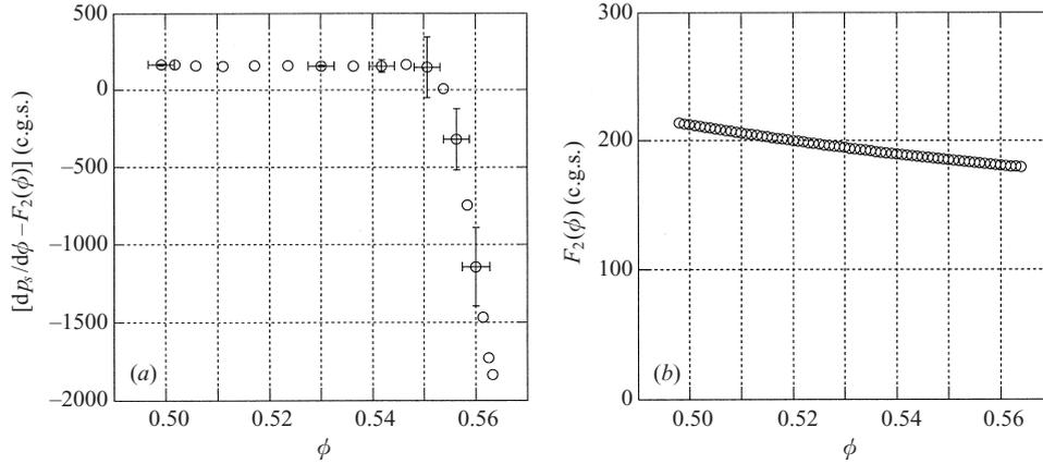
FIGURE 21. (a)  $[dp_s/d\phi - F_2(\phi)]$  as a function of  $\phi$  for the wave of combination 2 with  $\phi_0 = 0.538$ ; (b)  $F_2(\phi)$ , computed with  $C = \frac{1}{2}$ , for the wave of combination 2 with  $\phi_0 = 0.538$ .
