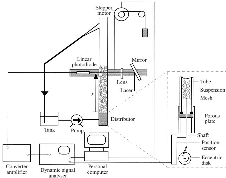
FIGURE 1. Sketch of the fluidized bed apparatus.
