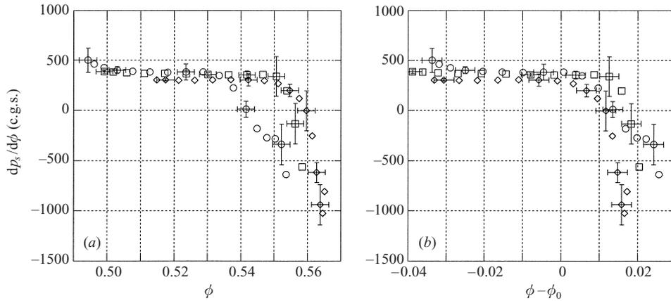
FIGURE 22. Influence of the mean particle concentration  $\phi_0$  on  $dp_s/d\phi$ : (a)  $dp_s/d\phi$  for combination 2 as a function of  $\phi$ ; (b)  $dp_s/d\phi$  for combination 2 as a function of  $\phi - \phi_0$ .  $\diamond$ ,  $\phi_0 = 0.548$ ;  $\square$ ,  $\phi_0 = 0.538$ ;  $\circ$ ,  $\phi_0 = 0.528$ .
