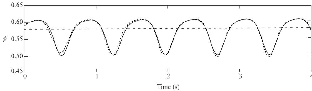
FIGURE 15. Example of a saturated wave fitted by a B-spline function. The saturated wave was obtained for combination 1 with  $\phi_0 = 0.57 \pm 0.005$  and  $f_0 = 1.4$  Hz. The dashed line is the experimental result and the solid line is the fitting B-spline function.
