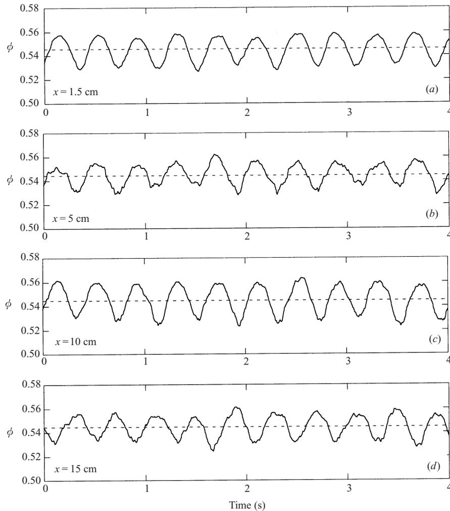
FIGURE 6. Spatial evolution of a neutral mode. This neutral mode was obtained when using combination 1 of particles, fluid and tube, with  $\phi_0 = 0.545 \pm 0.005$  and  $f_0 = 2.6$  Hz. The wave shape was measured at different positions  $x$  along the bed and obtained by averaging over 30 time sequences.
