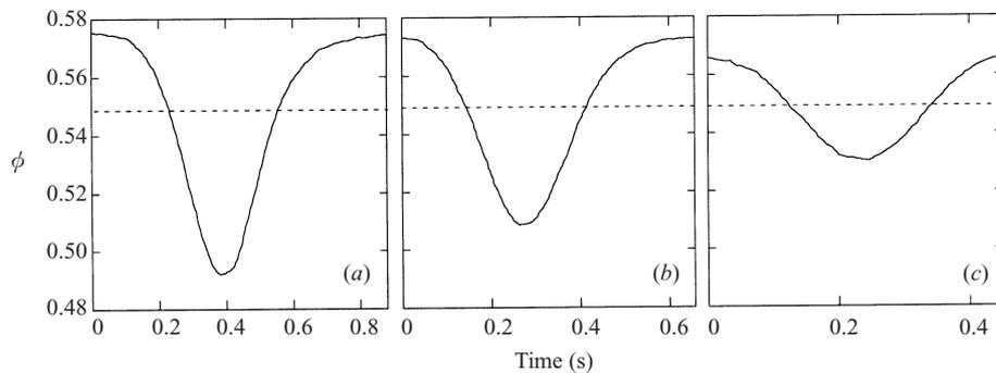
FIGURE 12. Influence of the forcing frequency  $f_0$  on the shape of the saturated wave: (a)  $f_0 = 1.1$  Hz; (b)  $f_0 = 1.55$  Hz; (c)  $f_0 = 2.2$  Hz. These waves were obtained with combination 6. Only one period of the wave is shown. The mean particle concentration  $\phi_0$  is  $0.549 \pm 0.003$  for the three waves. The dashed line shows the mean particle concentration  $\phi_0$ .
