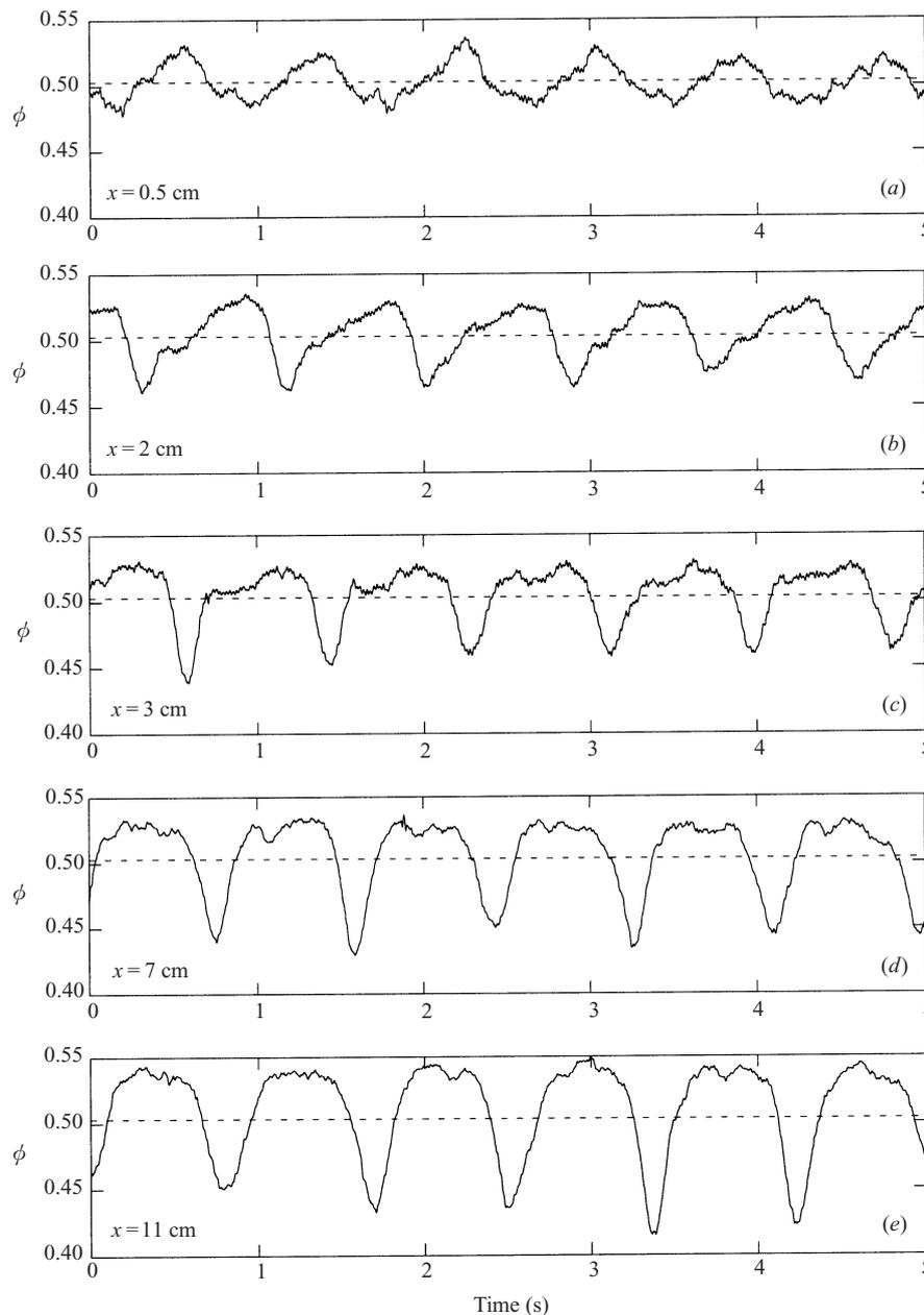
FIGURE 7. Spatial evolution of an unstable mode. This unstable mode was obtained when using combination 7 of particles, fluid and tube, with  $\phi_0 = 0.503 \pm 0.002$  and  $f_0 = 1.17$  Hz. The wave shape  $\phi$  was measured at different positions  $x$  along the bed and obtained by averaging over 30 time sequences.
