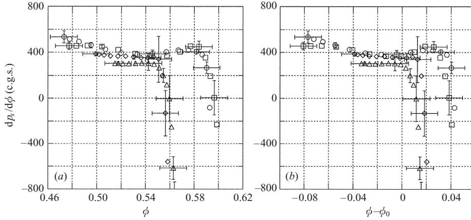
FIGURE 24. Influence of the fluid viscosity  $\mu_f$  on  $dp_s/d\phi$  : (a)  $dp_s/d\phi$  plotted against  $\phi$ ; (b)  $dp_s/d\phi$  plotted against  $\phi - \phi_0$ .  $\triangle$ ,  $\phi_0 = 0.548$ ;  $\diamond$ ,  $\phi_0 = 0.538$ : combination 2 with  $\mu_f = 3$  cP.  $\square$ ,  $\phi_0 = 0.558$ ;  $\circ$ ,  $\phi_0 = 0.55$ : combination 1 with  $\mu_f = 0.9$  cP.
