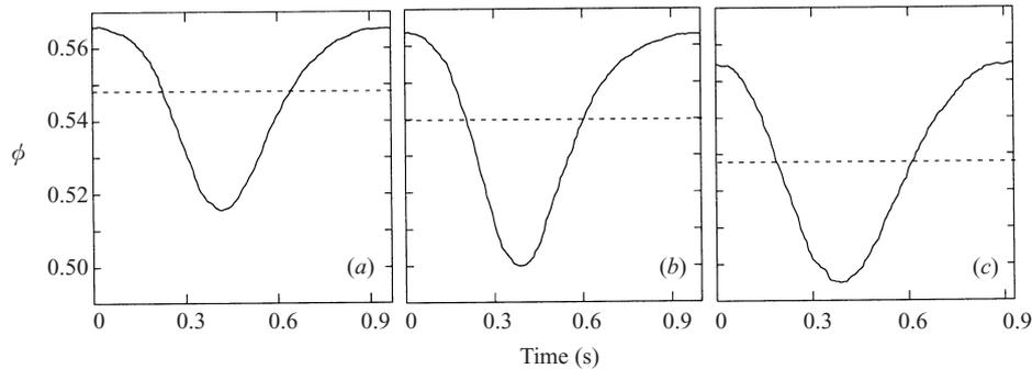
FIGURE 11. Influence of the mean particle concentration  $\phi_0$  on the shape of the saturated wave: (a)  $\phi_0 = 0.548$ ; (b)  $\phi_0 = 0.540$ ; (c)  $\phi_0 = 0.528$ . These waves were obtained with combination 2. Only one period of the wave is shown. The forcing frequency  $f_0$  is  $\approx 1.1$  Hz for the three waves. The dashed line shows the mean particle concentration  $\phi_0$ .
