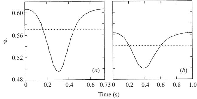
FIGURE 13. Influence of the fluid viscosity  $\mu_f$  on the shape of the saturated wave: (a) wave of combination 1:  $\phi_0 = 0.57$ ,  $f_0 = 1.4$  Hz,  $\mu_f = 0.9$  cP; (b) wave of combination 2:  $\phi_0 = 0.54$ ,  $f_0 = 1$  Hz,  $\mu_f = 3$  cP. The dashed line shows the mean particle concentration  $\phi_0$ .
