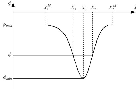
FIGURE 14. A saturated wave period plotted as a function of  $X$ . The quantities  $\phi$ ,  $\phi_{max}$ ,  $\phi_{min}$ ,  $X_0$ ,  $X_1$  and  $X_2$  introduced in §4.2 are shown.
