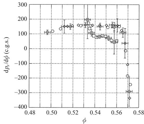
FIGURE 23. Influence of the forcing frequency  $f_0$  on  $dp_s/d\phi$ :  $dp_s/d\phi$  for combination 6 as a function of  $\phi$ .  $\circ$ ,  $f_0 = 1.1$  Hz;  $\diamond$ ,  $f_0 = 1.55$  Hz;  $\square$ ,  $f_0 = 2.2$  Hz.
