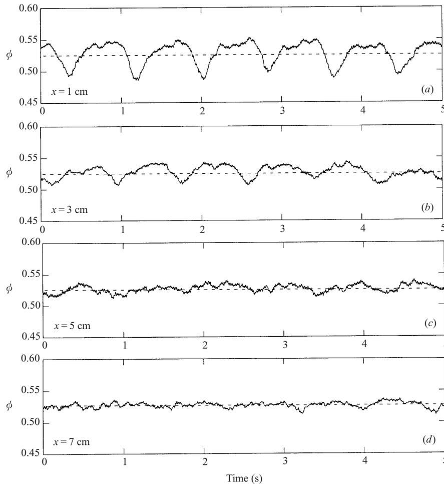
FIGURE 5. Spatial evolution of a stable mode. This stable mode was obtained when using combination 7 of particles, fluid and tube, with  $\phi_0 = 0.524 \pm 0.002$  and  $f_0 = 1.22$  Hz. The wave shape was measured at different positions  $x$  along the bed and obtained by averaging over 30 time sequences.
