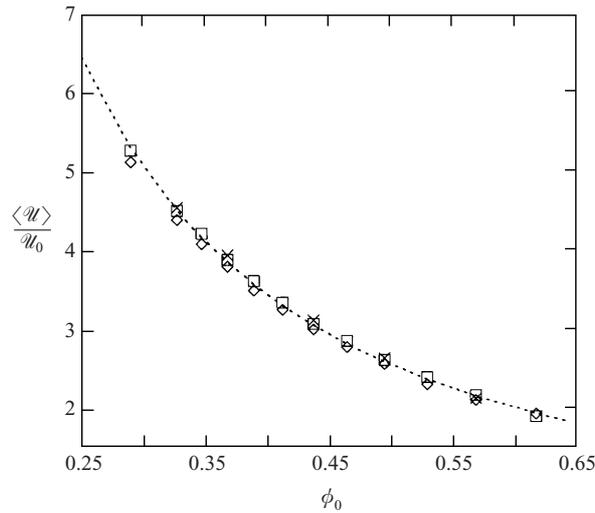
FIGURE 2. Calibration of the averaged signal,  $\langle \mathcal{U} \rangle$ , with the mean volume fraction,  $\phi_0$  at  $\diamond$ ,  $x = 5$  cm;  $\square$ , 10 cm;  $\times$ , 15 cm. The dotted curve corresponds to the best power law correlation,  $\phi_0^{\zeta}$  with  $\zeta = -1.35$  for combination 6.
