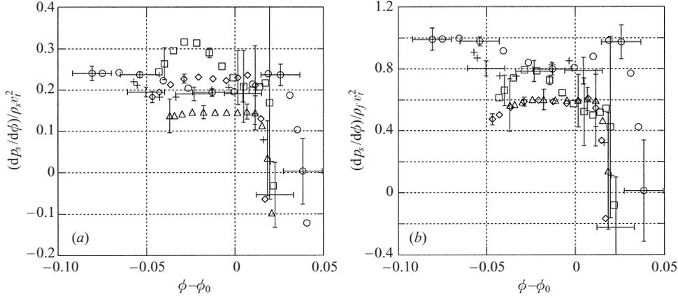
FIGURE 27. Scaling laws for  $dp_s/d\phi$ : (a)  $(dp_s/d\phi)/\rho_s v_t^2$  as a function of  $\phi - \phi_0$  for a representative sample of curves; (b)  $(dp_s/d\phi)/\rho_f v_t^2$  as a function of  $\phi - \phi_0$ .  $\circ$ ,  $\phi_0 = 0.558$ , combination 1;  $\square$ ,  $\phi_0 = 0.545$ , combination 3;  $\times$ ,  $\phi_0 = 0.527$ , combination 4;  $\triangle$ ,  $\phi_0 = 0.549$ , combination 6;  $\diamond$ ,  $\phi_0 = 0.530$ , combination 8.
