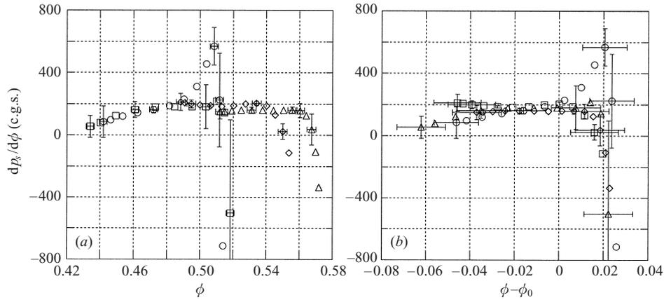
FIGURE 25. Influence of the bed to particle ratio  $D/d_s$  on  $dp_s/d\phi$ : (a)  $dp_s/d\phi$  plotted against  $\phi$ ; (b)  $dp_s/d\phi$  plotted against  $\phi - \phi_0$ .  $\circ$ ,  $\phi_0 = 0.488$ ;  $\square$ ,  $\phi_0 = 0.496$ : combination 7 with  $D/d_s \approx 10$ .  $\triangle$ ,  $\phi_0 = 0.549$ ;  $\diamond$ ,  $\phi_0 = 0.534$ : combination 6 with  $D/d_s \approx 25$ .
