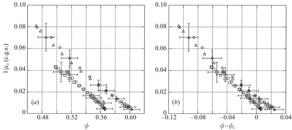
FIGURE 17. Influence of the fluid viscosity  $\mu_f$  on  $\mu_s$ . (a)  $1/\mu_s$  plotted against  $\phi$ ; (b)  $1/\mu_s$  plotted against  $\phi - \phi_c$ ;  $\circ$ ,  $\phi_0 = 0.548$ ;  $\square$ ,  $\phi_0 = 0.538$ : combination 2 with  $\mu_f = 3$  cP and  $\phi_c = 0.560$ .  $\diamond$ ,  $\phi_0 = 0.558$ ;  $\triangle$ ,  $\phi_0 = 0.55$ : combination 1 with  $\mu_f = 0.9$  cP and  $\phi_c = 0.578$ .
